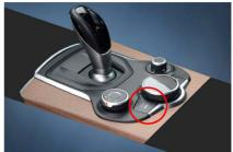
Switch using the "MENU" key. Switch back to OE using any button. It will automatically go back to OE screen.
