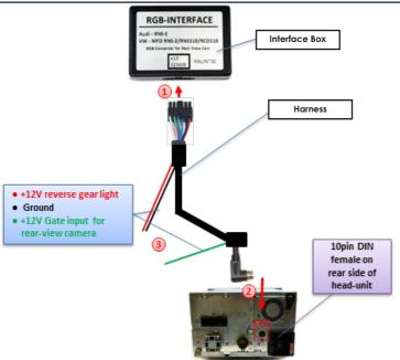
NB: If the female 10pin DIN-connector of the head unit is already occupied, the vehicle has a factory TV-tuner. In this case it must be uninstalled. Disconnect the male 10pin DIN-connector of the factory harness and disconnect all wires from the factory TV-tuner.
