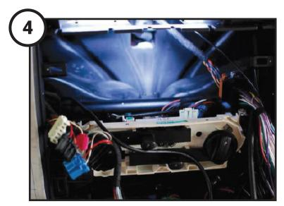
Remove the metal clips and reroute the air vent wiring
