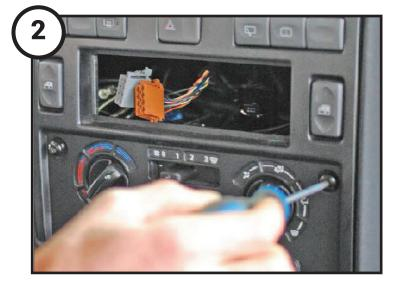
Remove the T-30 screws from the main OEM fascia panel
