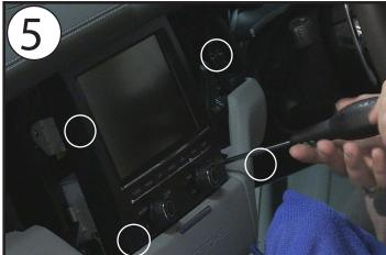
Use a screwdriver to remove the four screws surrounding the OEM display.
