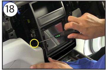
Secure the fascia panel to the cage with one screw on each side of the assembly.
