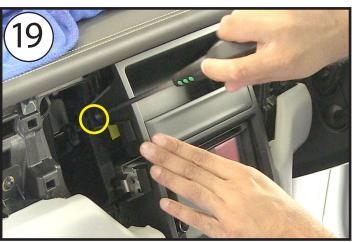
Secure the fascia panel to the dashboard using the two top screws removed during Step 5.
