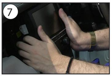
Ensure that the gear shifter is covered by an appropriate protective material and put it into reverse to allow space for the OEM display and head unit to slide out.
