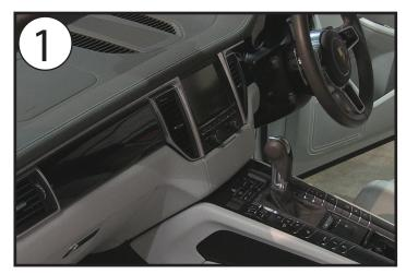
Porsche Macan OEM dashboard. Ensure that appropriate areas of the dashboard are protected by suitable material to avoid damage or scuffing during the installation.
