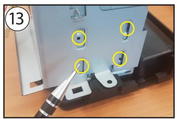
Once properly seated into position, screw the cage onto the head unit on each side (4 per side) using the x8 included Hex screws.
