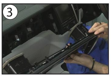
Once unclipped, pull out and remove the trim panel and both passenger-side air vents. Store the piece safely for reassembly.
