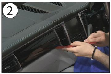
Firstly, unclip the trim panel on the passenger side of the dashboard using a panel removal tool. Pry using a panel removal tool at the location highlighted in the image. The panel will begin to come away with the air vent on the far side, and the one next to the OEM display.
