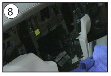
The dashboard will now be completely stripped of the OEM head unit and display and the aftermarket kit can be assembled and installated.
