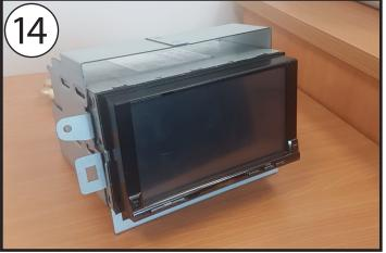
After this step is completed, the new head unit and cage assembly will be finished and this can be installed into the factory dashboard.
