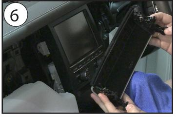
Pull the 'Porsche' branded trim piece away from the dashboard by hand. Note that the piece was being held in place by the black plastic brackets (unscrewed in Step 5 - bottom corners) so lift and pull to remove the trim.
