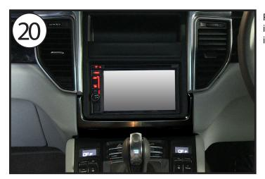
Reinstall all other dash components including the vents in the reverse order of disassembly to complete the installation
