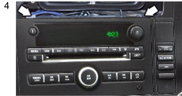
Remove the 2 screws as indicated. then pull out the head unit.
