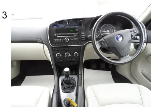
Remove the centre air vent
