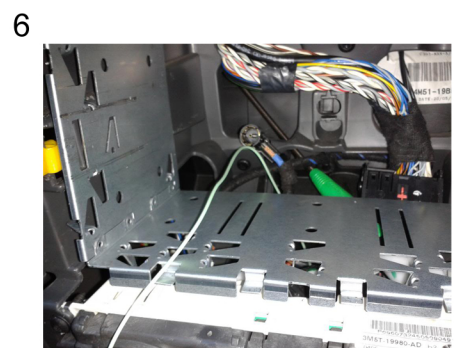
Push in the metal clip to secure the cage into place.
