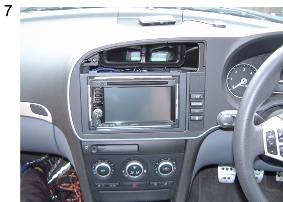
Fit the head unit into the cage, then fit the replacement panel.
