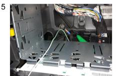
Push in the metal clip to secure the cage into place.
