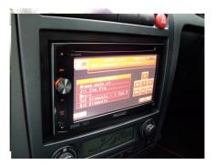
Fit the head unit into the cage, then fit the replacement panels.
