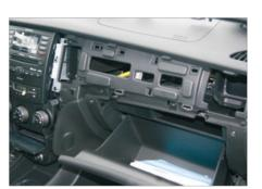
7. Remove whole panel with integrated air vents
