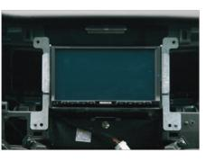
Attach metal mounting brackets to Double-DIN navigation
