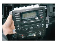
Remove screws of OEM-head unit. Remove OEM head unit by pulling it towards your direction
