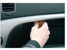
2. Open glove box - remove two screws beneath silver panel
