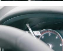
Remove 2 screws beneath tachometer unit cover left and right side
