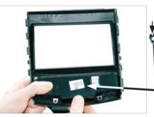
10. Remove OEM panel holding harzard light switch and clock.
