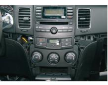
3. Unclip and remove silver panels at left and right side carefully
