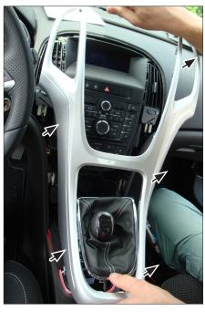
2. Remove screws of OEM center panel
