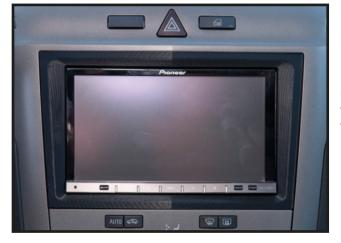
Connect all of the wiring to the stereo and slot into the cage (already installed into the dashboard). Test the radio and proceed to finally place the new fascia plate over top to finish the installation.
