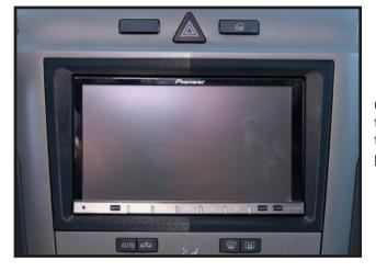
Connect all of the wiring to the stereo and slot into the cage (already installed into the dashboard). Test the radio and proceed to finally place the new fascia plate over top to finish the installation.
