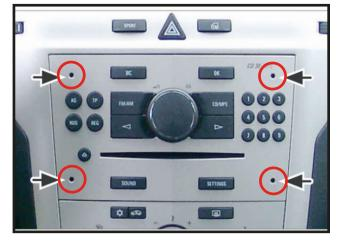
Begin by using a set of radio removal keys in the following holes to release the main head unit. Once released, pull the radio forward and disconnect all of the wiring.
