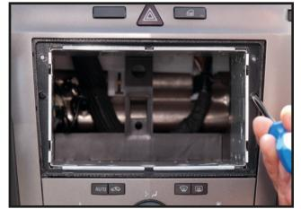
Attach the mounting frame into the dashboard and screw into place (screws not supplied).
