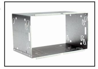
Take the cage within the kit and proceed to push into the dashboard opening once the mounting frame has been fitted. Once seated correctly, bend all the tabs either side to fix into place.
