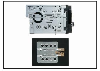
Take the mounting brackets that come within the kit and arrange them onto the relevant sides of the radio as shown in the image. The position/alignment of these brackets can be adjusted for the "perfect fit".
